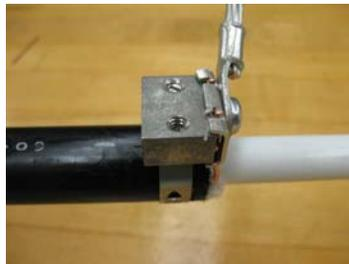
Figure 3 – Alternative method for attaching equipment conductors.
